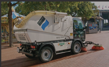
First vacuum sweeper multiservice vehicle model B300/400H
